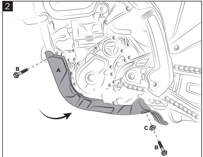
**Position the fuel tank Acerbis (A) and screw first in front with two screws (B) without tightening them, then the other two screws (B) at the rear with the bushings (C) supplied. Finally close and tight all four the screws.**
